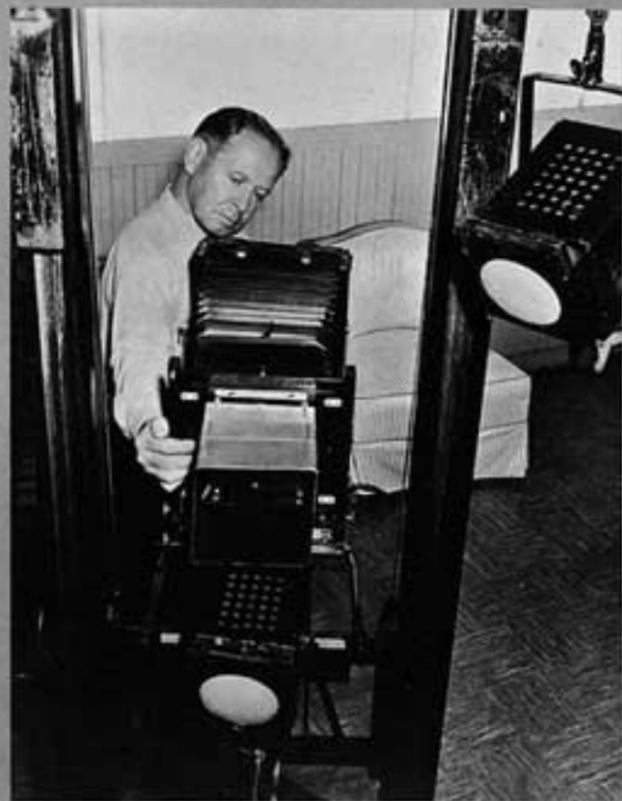
Massive twin-parallel camera stands, like the ones featured in this picture of C. S. Bull, were the rule, rather than the exception, in Hollywood. Like a modern pillar-type stand, they allow the camera to be lowered almost to ground level, or raised well above eye level, quickly and smoothly.
