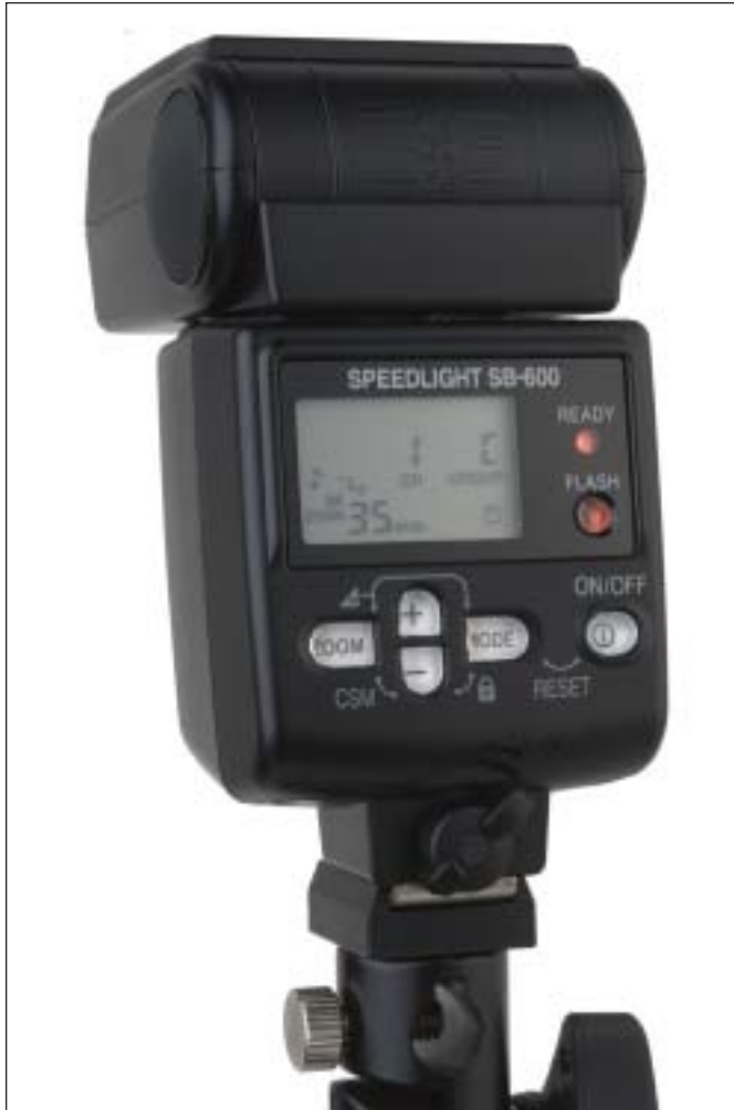
The rear of the SB-600 shows that it is a simpler flash to use than the SB-800. Though it is about 20 percent less powerful than its bigger sibling it makes up for the lack of power by having a reduced recycle time and by getting more life from its batteries. Note that this particular flash is set up in the “remote” mode.
