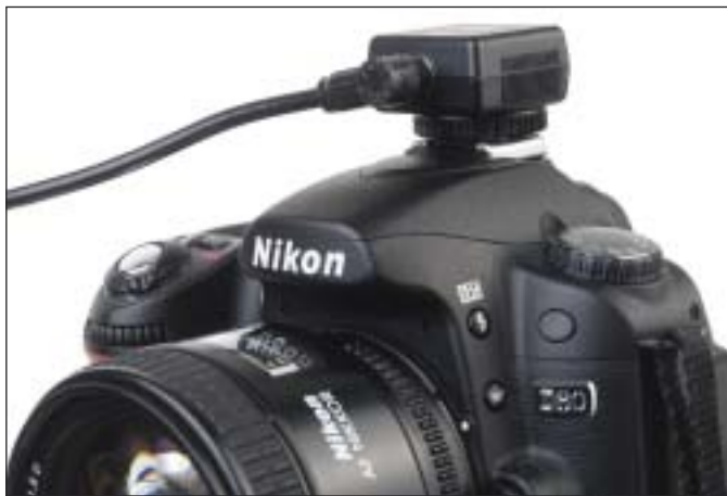
The Nikon D80 digital camera is a model that lacks a built-in PC connection. The D80 is shown here with the Nikon AS-15 hot shoe-to-PC accessory connected to a standard synchronization cable.
