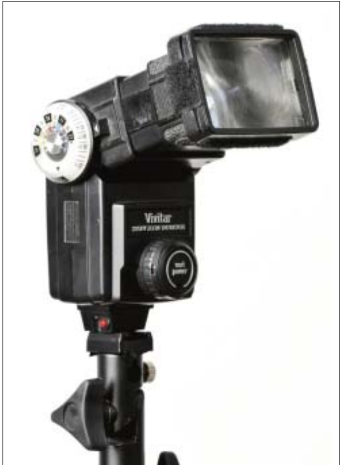
Vivitar 285 HV. This side view shows off the Vivitar 285’s zoom head feature as well as the lighted white dial that allows quick automatic and manual settings. The “HV” in the name referred to its ability to be used with dedicated high-voltage, external battery packs.
