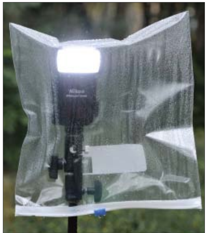
Splashproofing your flash. The handy one-gallon-sized plastic kitchen bag makes a perfect raincoat for flashes that can triggered either by infrared or via radio remote. No reason to stop shooting in a light rain. But I'd never risk shooting an A/C powered strobe under rain conditions!
