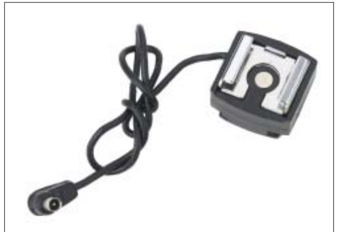
This is a generic accessory called a PC-to-hot shoe adapter, available at most photo retailers, that allows you to connect a radio slave or any other PC socket-terminated device to a flash that lacks a PC socket.
