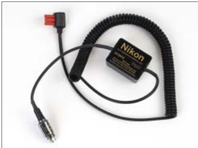
This is a specialized connecting cord for mating a DCB HV battery module with the high-voltage socket of a Nikon SB series flash. The small box on the connecting cord contains electronics that limit the recycle speed to ensure that the flash doesn't overheat and get destroyed. I've used one for three years without losing a single flash unit.
