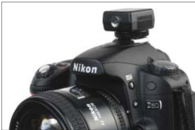
The Nikon AS-15 connector is an adapter that sits in the hot shoe of a camera and provides a standard PC sync socket for cameras that lack them. It can be used with all popular brands and models of cameras with the exception of the Sony and Minolta lines of SLRs. Those cameras use a proprietary hot shoe design.
