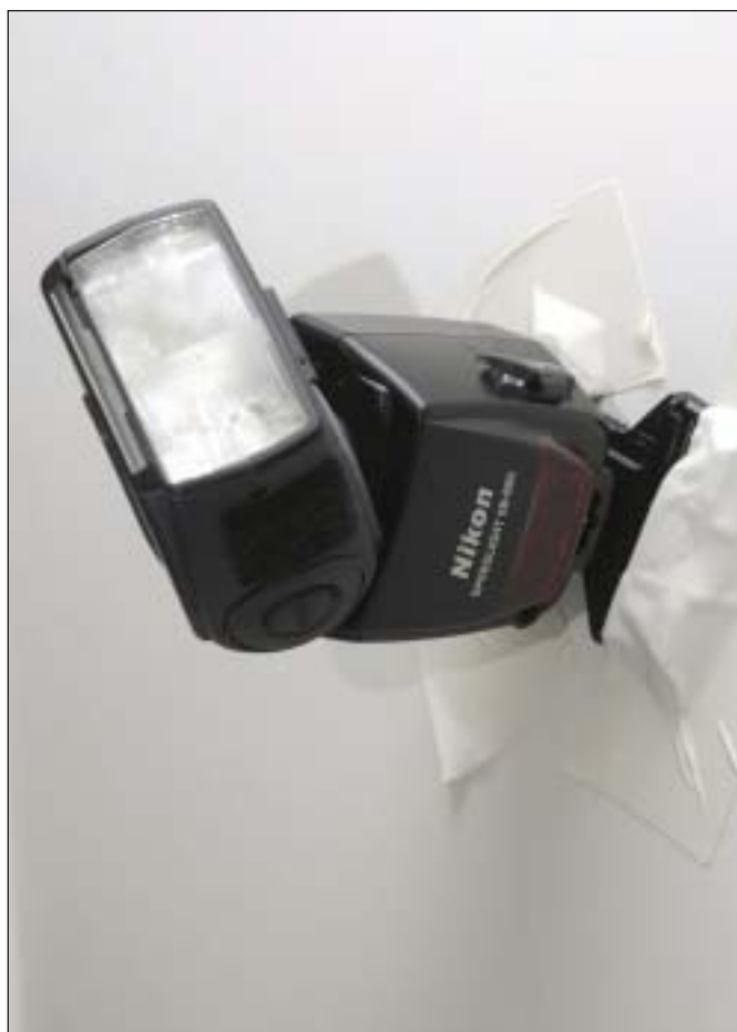
The Nikon AS 19 flash adapter offers a wide "lip" that makes it practical to attach a flash unit to just about any flat surface. Shown here anchoring an SB-800 to a door with a liberal application of gaffer's tape.
