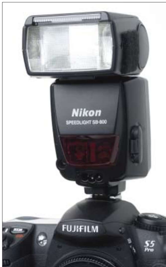
The Nikon SB-800 is the current top-of-the-line flash in the Nikon system. Used in its commander mode it can control up to three groups of flashes. Its preflash systems is the current champion for correct exposure control. It is smaller and more powerful than its predecessors. Shown here mounted to the new Fuji S5 Pro digital camera it provides the Fuji product with the same range and features as the Nikon cameras.
