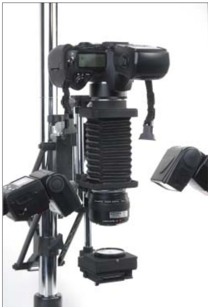
Close-up of my macro rig with SU-800 flash controller providing wireless TTL flash in conjunction with my D2x camera. This combination of camera and lens can shoot at up to 10x life size on my reduced-size sensor.
