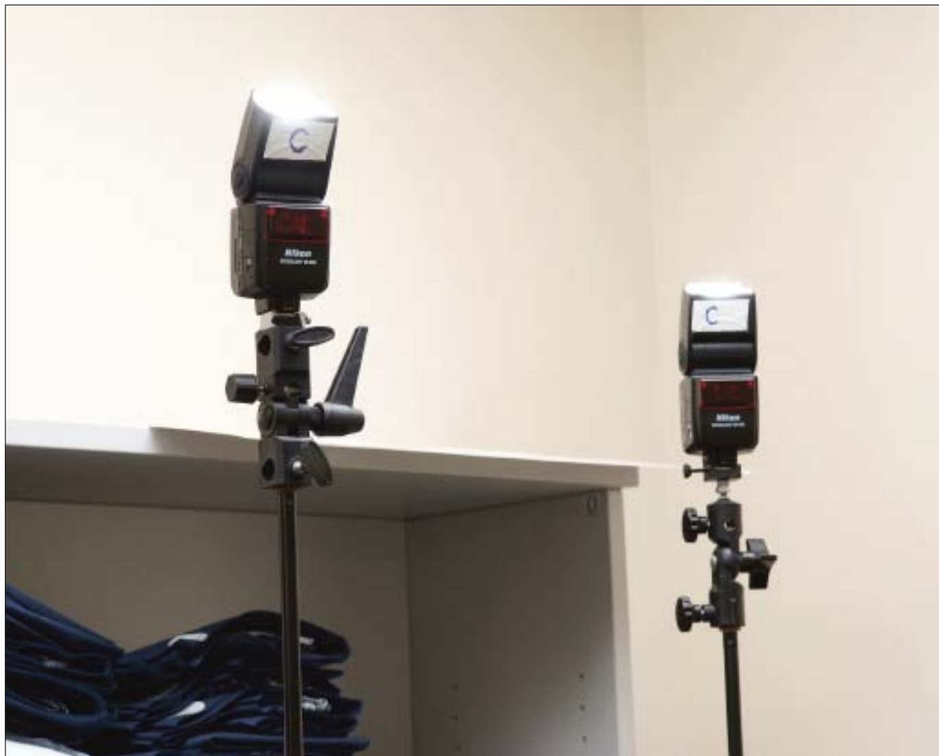
We often use wirelessly controlled lights bounced from white ceilings to provide a soft even fill light for interior locations. Shown are two Nikon SB-600 units. All of our Nikon flashes have been assigned specific groups. Notice the letter C on the gaffer's tape. Both of these flashes are controlled by a master flash.
