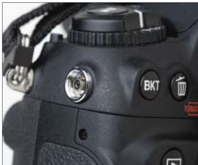
One standard in all professional-caliber digital and film cameras is the inclusion of a standard PC socket for studio flash connection. Shown here is the PC socket on the latest Fuji S5 Pro camera.
