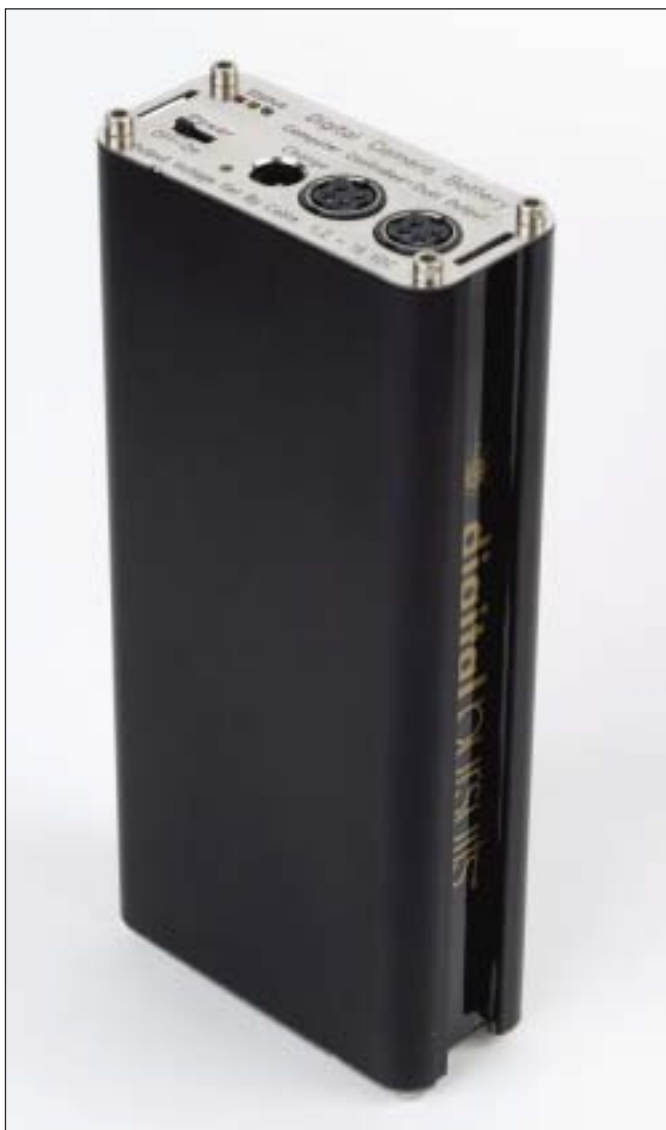
A Digital Camera Battery DCB-40 external battery pack. This high-voltage battery supplies 320 volts and plugs into the HV ports of most professional flash units. It can recycle most flashes at nearly 1 fps. The company supplies cords for several flashes that slow down the recycle times to keep from burning out the flash unit's tube or electronics. The advantage over a lower voltage pack is speed, speed, speed. The HV port of most flashes bypasses the charging circuitry and applies power directly to the capacitors. If you use a high-voltage battery pack with your TTL flash, you'll still need to use the internal AA batteries to run the exposure electronics!
