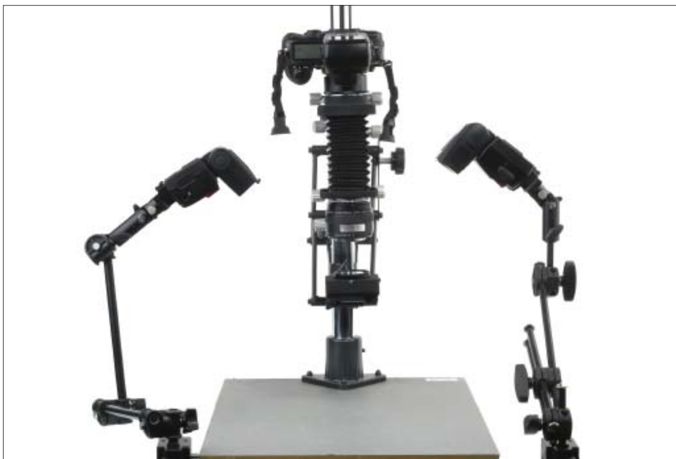
Macro rig with TTL lighting control. My business often is called on to document tiny products from the high-tech business segment. Our macro rig consists of a PB-4 bellows, an Olympus 35mm macro lens, a PS-4 slide stage, and a copy stand. Our lighting comes from two SB-600s triggered by an SU-800 flash controller mounted on a Nikon D2x. I need to be able to precisely position our lights and then leave them in position for a long time. I depend on articulated arms coupled with Alzo stand adapters secured to the tabletop with Manfrotto Super Clamps.
