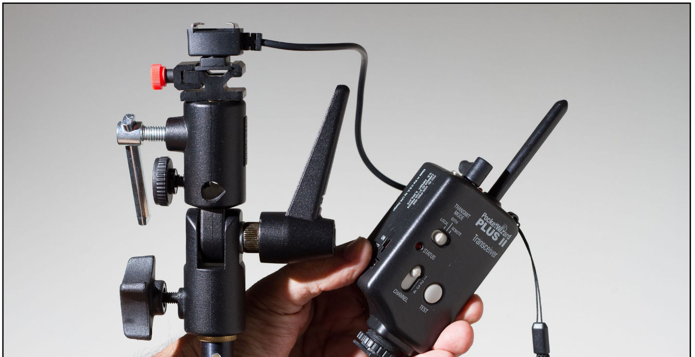
Figure 8: In some configurations, a hot shoe to PocketWizard adapter is also attached.
