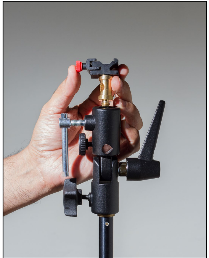
Figure 7: Screw the stud (this one comes with the Manfrotto brand umbrella adapter) to the cold shoe and attach it to the umbrella adapter.
