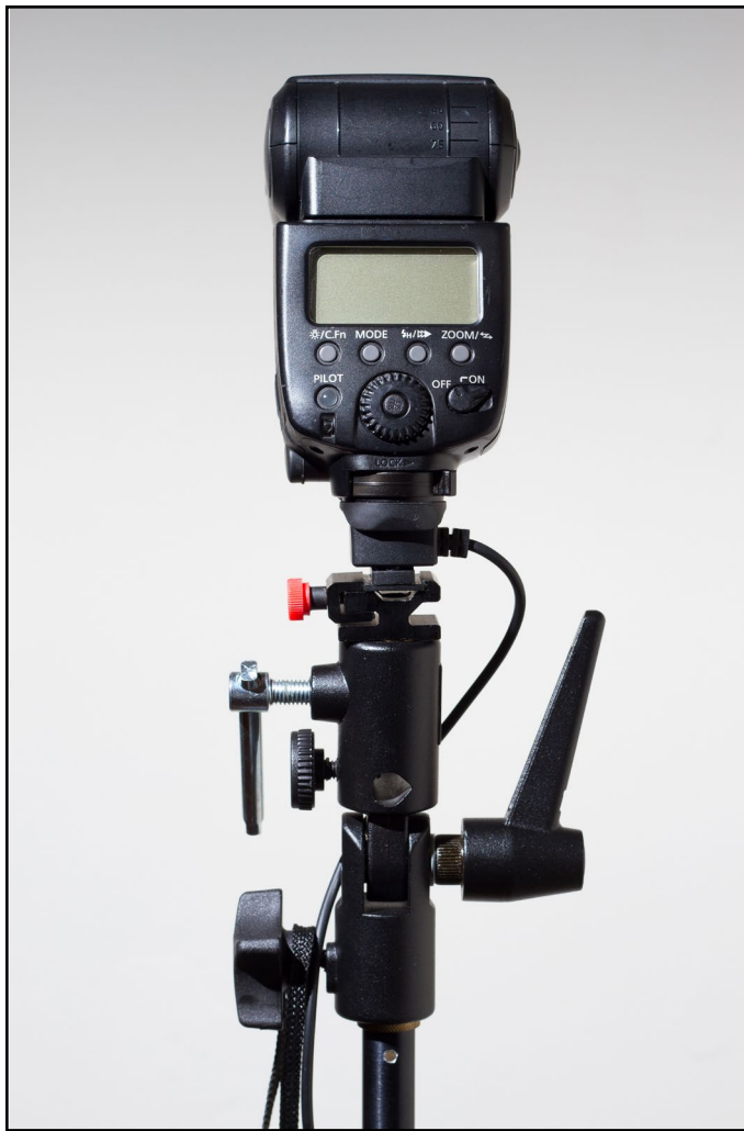
Figure 9: Attach the flash unit to the stand. PocketWizard adapter shown here.
