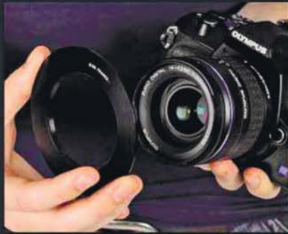
1) Screw in the appropriate adapter ring
