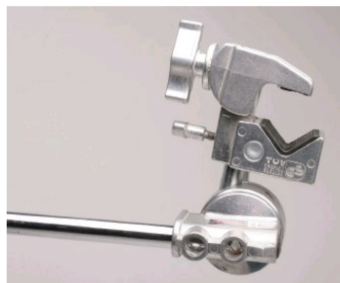
Figure 6.18: Grip arm with a super clamp. The super clamp has a “v” shape on the bottom, which holds anything that is round such as a pole, light stand, PVC pipe, and so on.
