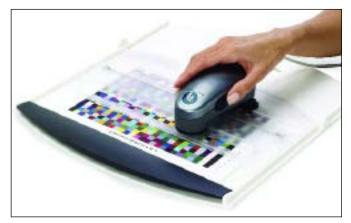
The GretagMcBeth Eye One spectrophotometer comes with a convenient ruler guide and backing board so that the colored wedges of the test print can be read quickly and accurately. The data is then processed to create an ICC profile that gets loaded into the computers that are printing to a specific printer with the profiled paper.
