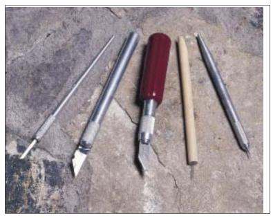
Basic retouching tools include abrading tools (left) and print abrading tools (middle) as well as an etching knife (right). All are used to reduce density or imperfections on the negative or print. Photos on this page by Bill Hurter.
