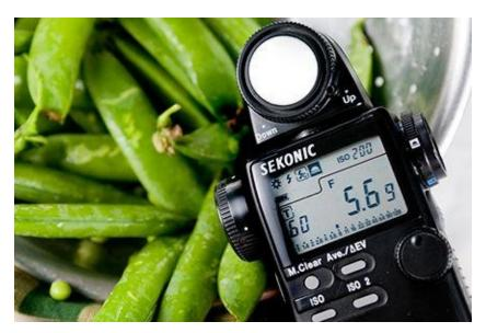
Figure 9-16: A hand-held light meter measures light reflecting off and falling on a subject.
